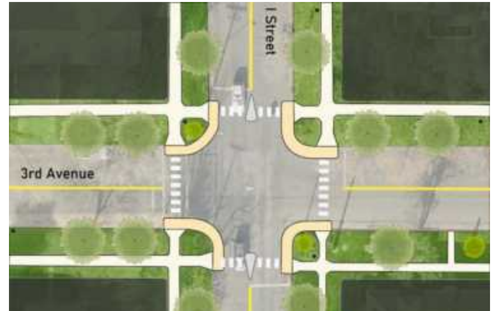
A redesigned 3rd Avenue and I Street intersection in the Avenues that incorporates pedestrian islands, curb extensions, and improved lighting to calm traffic and increase safety. These features reduce crossing distances, slow turning vehicles, and improve visibility at a steep and often fast-moving intersection.
