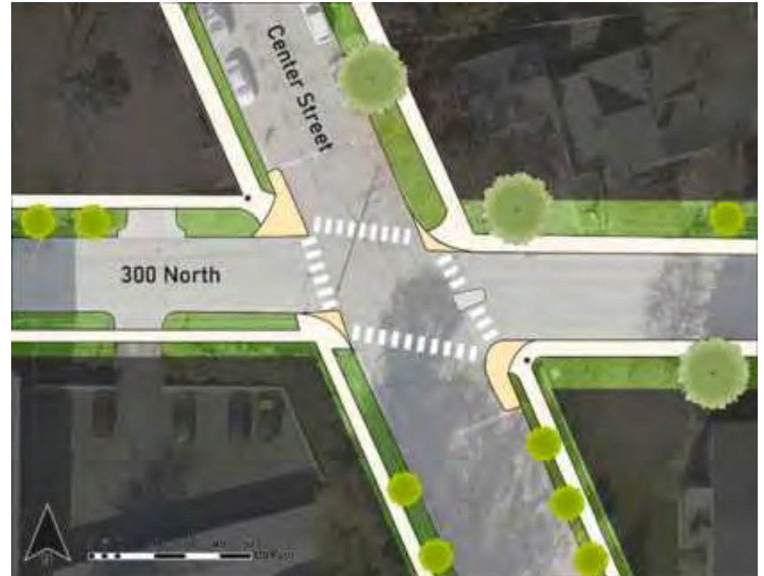
A potential redesign of the 300 North and Center Street intersection in Capitol Hill, featuring pedestrian islands, curb extensions, and added lighting to improve safety and visibility. The design shortens crossing distances, formalizes existing driver behavior caused by steep slopes, and encourages slower, more cautious turns.
